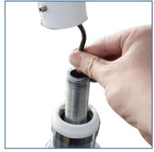
7. Adjust the direction of the phoroptor arm to be perpendicular to the main machine, use an Allen key to lock the screw which are inside the arm.
