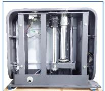
3. Remove the two screws fixed on the tray (as shown in the figure below), lift the main machine and place it on the ground, then adjust the four foot pads for stable placement.
