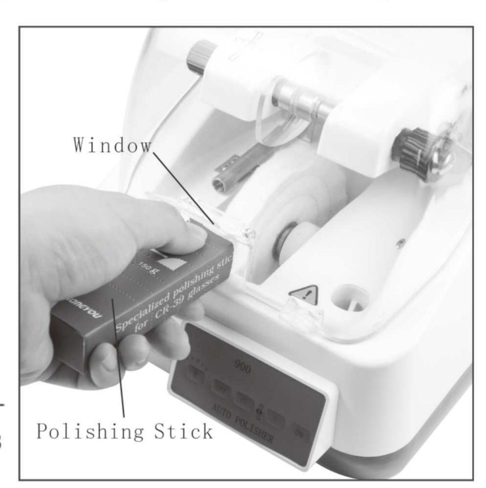
Using the position control knob, you can slide the lens to an appropriate place against the buffing wheel at any time.
