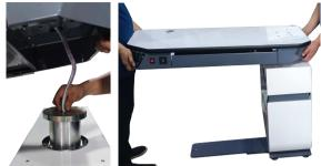
6. Align the screw holes and put the large table-top down, screw in 4 innerhexagon screws (M10) and cover them with silicone blockings;
