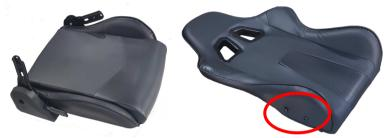
3. Install the backrest as shown in the below, cover the plastic parts after tightening the screws, and repeat above operation on the other side;
