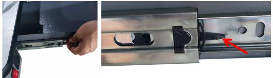
9. Place the small table-top as shown, align the slider below with the screw holes and screw in 4 screws;
